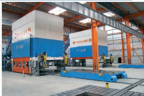
N.2 PDM-4B-E-1000 TABLE SIZE 5000x2500 mm.
