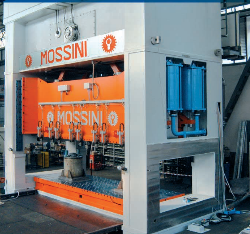
PDM-4B-LD-1250 TABLE SIZE 6300x2000 mm.
